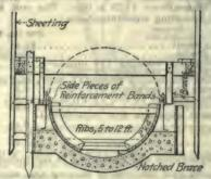
Fig. 21.—Concrete Sewer Construction.
